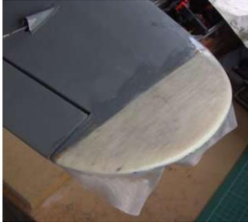
The original wing tips were hollow, but new ones were just made from thick sheet, sanded to shape and covered in glass fibre faired into the existing covering.
