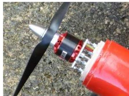
With the motors connected and the cabling complete, a directional check was carried out. Both motors turn in the same direction. A power check was carried out with 9X6 electrical props and the system was drawing in excess of 60 amps and 700 watts, this
