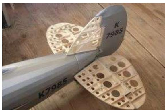
Secondly, the tail surfaces were originally covered in Litespan, which is not very tough and had acquired several holes. The polyurethane varnish has also yellowed badly. So tail surfaces have been stripped back to the wood and will be covered in Solartex like the rest of the model. The slight extra weight will be compensated for by a couple of ounces of lead in the nose, which is not a problem as the model is quite light already.
