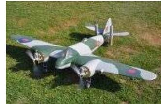
I also noticed a little chattering on some servos, which I eventually realised was due to glitches on the 35MHz aerial. The model has two sets of pull-pull cables (rudder & tail wheel) and a servo cable (tail wheel retract) running down the fuselage parallel to the aerial, so not really surprising. A change to 2.4GHz has fixed this, and taking Dave's point about 6v batteries, the heavier battery has given a bit more nose weight.
