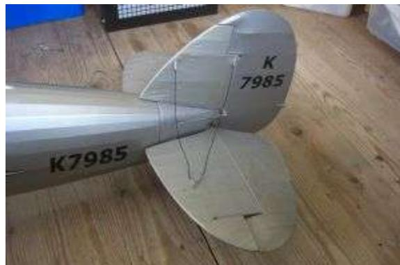
Firstly, the rigging, which was done using elastic thread, had gone very limp. This has now all been replaced by nylon-covered steel wire for the fuselage and tail bracing, and nylon fishing line for the wing bracing, where some stretch is required.
