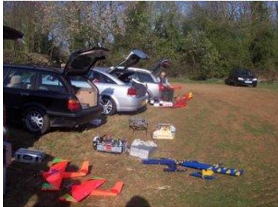
There are two basic plane designs – v tail (orange in photo) which fly better in knife edge but are harder to set up and fly smoothly – and standard tail (blue) which Mike and I fly. ARTF kits are available too. They come with either balsa or fibreglass fuselages. Fibreglass is quicker to build and more durable - but harder to repair!
