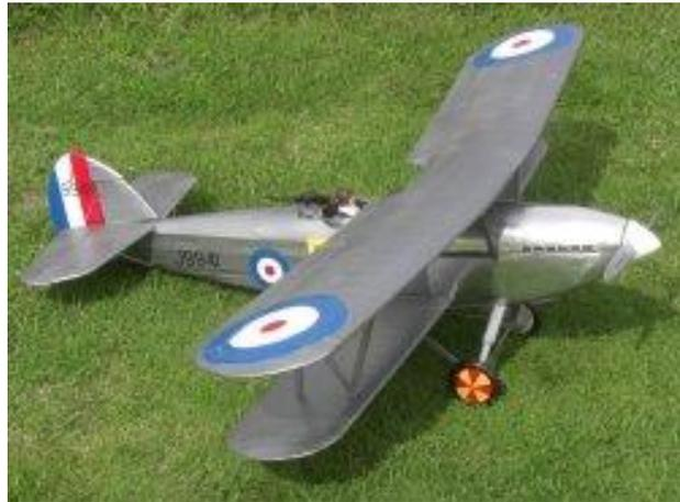
Covering was done in traditional form with tissue, nylon and dope, finished with a silver car paint spray. The nose area, which was aluminium panels on the full size, was covered in "Aluclad", a thin adhesive-backed aluminium foil. Rigging is from nylon fishing line. The main advantage over my larger biplanes is that this one will go in the car without disassembling it!
