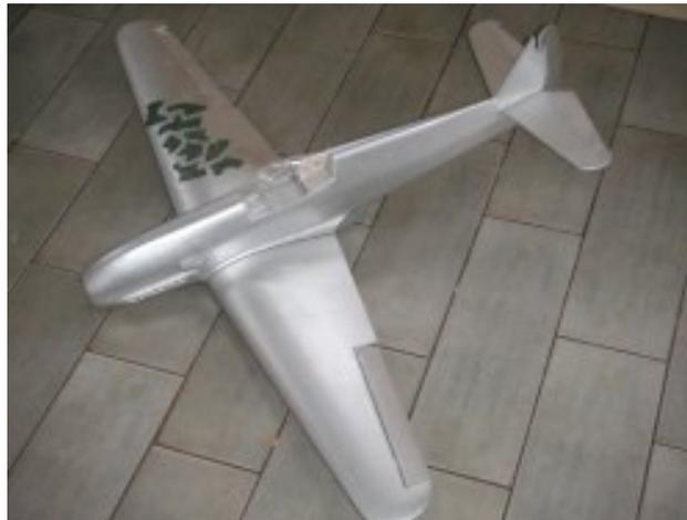
Details: 47" span, glass-covered foam wing, designed for 20-25-size engines and 4-function radio with small servos, hand-launched (or fit U/C, but see my comment about wheels above). Design weight 3 to 3.5 lbs, current airframe weight 1lb 11oz. Aluminium paint with camouflage started but not completed. Very tattered original plan and instruction booklet included.
