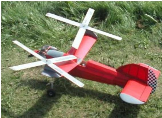
**Mike O'Leary's** twin-rotor autogyro flies quite well, but one or even both rotors can stop in flight as the wing takes the lift, which makes flying rather interesting...
