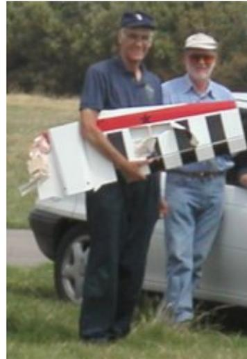
**Mike Barnett's** big Cap232 didn't fare too well when the wing gave way in the air. Soft balsa and lightweight construction commonly used in these ARTF models is suspected as the cause; the break was just past the end of the ply dihedral brace.
