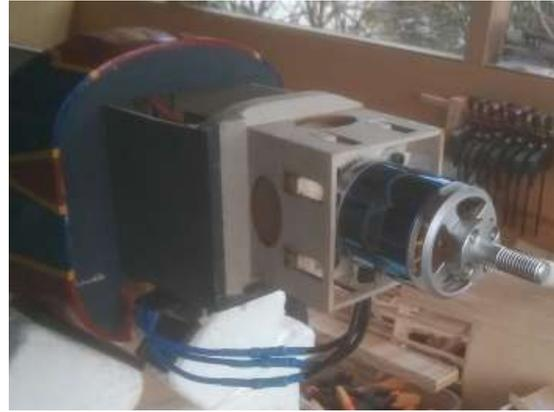
The hatch which takes up most of the very long front is attached with two bolts – fine for the IC version where access is only required to attach and remove the wings, but not for electric where access is required each flight. So I fitted magnets and a safety catch which allow it to be removed instantly but remain firmly closed in flight.
