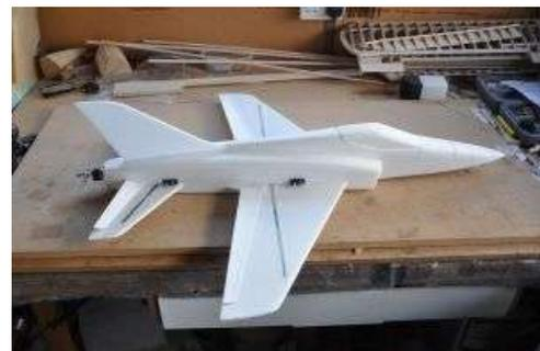
Construction is relatively easy; Depron cuts easily with a sharp knife or scalpel, and UHU POR contact glue or 5-minute epoxies are used to glue it. Carbon-fibre tubes are used to give the wing and tailplane strength.
