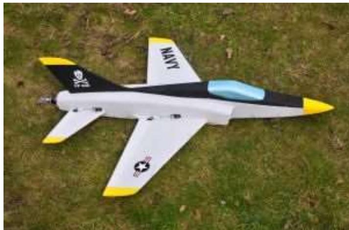
I finally got round to finishing the Bandit, painted in a US Navy style unashamedly copied from a model on the Internet. Acrylic paint was used brushed on, and the markings were cut from vinyl. In fact it was copied a little too closely, as the US marking should actually be on the left wing. Oh well...
