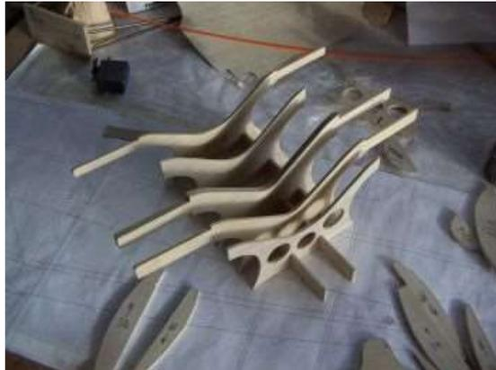
The ends of three of these sections engage with slots in the wing panel ends and the result is shown below ready for sheeting.
