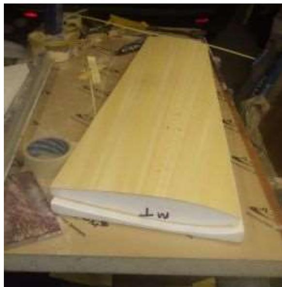
The construction has been shared, with Mike responsible for the wings and tails and Pete the fuselages. The wings are cut from foam and then covered in veneer (see later article). The fuselages are a fairly simple box construction with limited shaping required – with a little care they can be built straight and true without the need for a jig.
