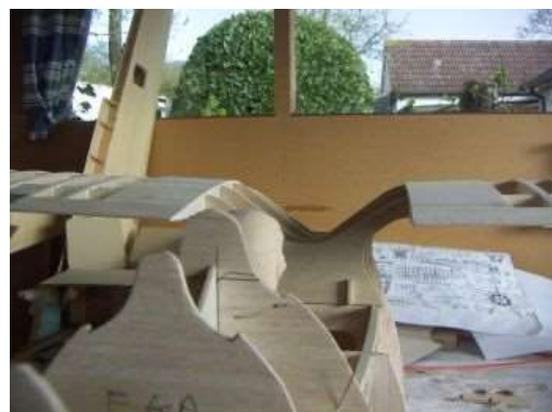
The fuselage is a box section with formers glued around to give the shape, then sheeted over the front part with stringers on the rest.
