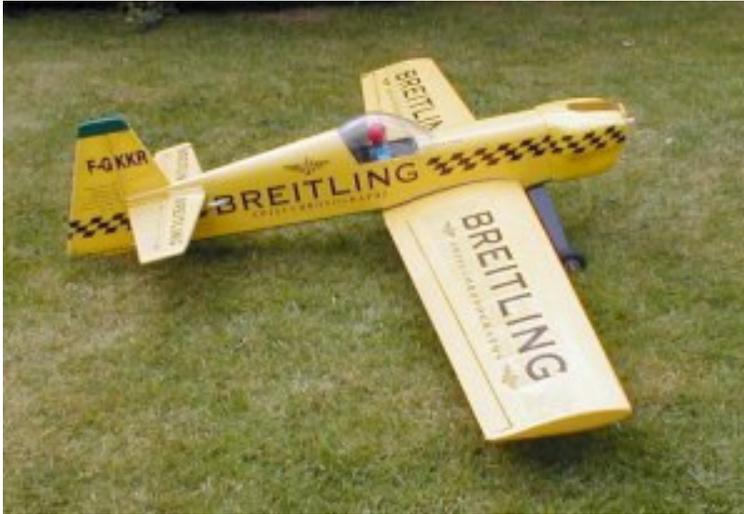
**VMAR Cap 231EX** semi scale sports model. Suitable for 40 - 53 two stroke (was flown with an Irvine 53).
