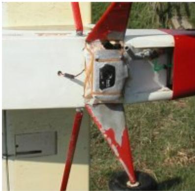
**Robin Thompson** mounted a cheap but effective film camera under his Precedent T240 with rubber bands and foam. A servo activates the shutter. With an ASP 120 4-stroke for power this model is capable of lifting even a heavy camera with ease. This camera only had a manual advance, so Robin had to land after each picture. He later fitted a camera with electric wind-on and was able to take multiple shots before landing.
