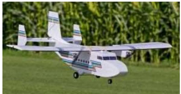
Power will be two 1220KV 133W motors which should be more than enough for an all-up weight of about two pounds. Prototypes are reported to go vertical in most un-cargo-like behaviour!
