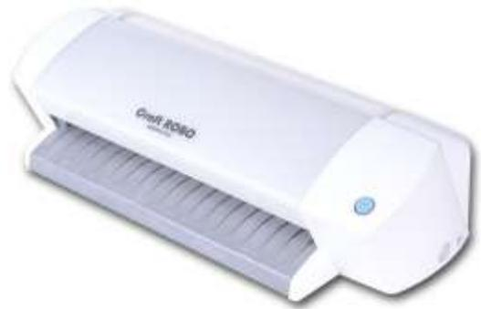
It's about the size and shape of a small PC printer and works in a similar way with a roller to move the paper back and forth and a carriage moving left and right. However this carriage holds not a printer head but a tiny knife blade which protrudes just a few tenths of a millimeter. This depth can be adjusted to cut film, vinyl or cardboard.
