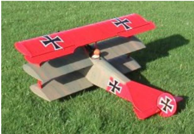
Fokker Tri-plane by **Trevor Hoskins**, from the Ripmax kit. Trevor has modified the kit quite a bit to make it more scale. Among the changes are a more accurate wheel spacing, which has improved ground handling, and a bigger cockpit.
