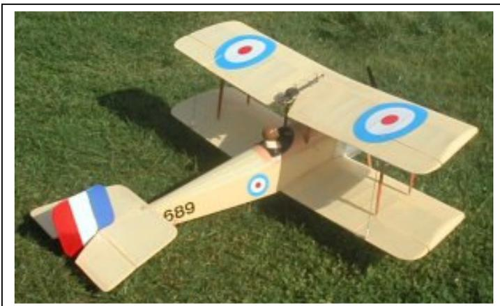
Nice Bristol Scout from the Svenson kit, by **Trevor Hoskins**. Flies well on a 46 2-stroke fitted with a dustbin silencer. Fully built-up construction, covered in "antique" Solartex.
