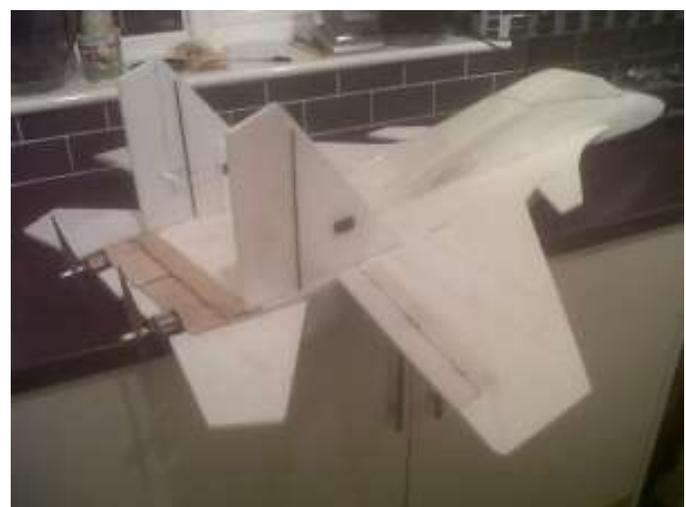
One last tip – add some wire triangle shaped ‘legs’ to the rear of the jet pipes – so that the props and tailerons are lifted clear of the ground – saves the props and stops the servos stripping their gears if you knock the tailerons on landing – ‘been there done that’ as they say.
