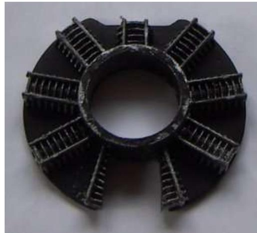
and painted. For dummy engines I first paint silver, let it dry thoroughly, then lightly spray with black which is wiped off immediately with a rag, giving a 'dirty metal' appearance.
