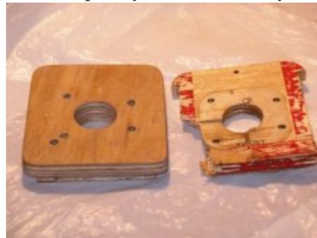
The remaining features, holes for fuel tubing, engine bearers and throttle connection, were marked out and drilled. In positioning the engine bearers, I compensated as best I could for the slight change in the vertical position of the new firewall.
