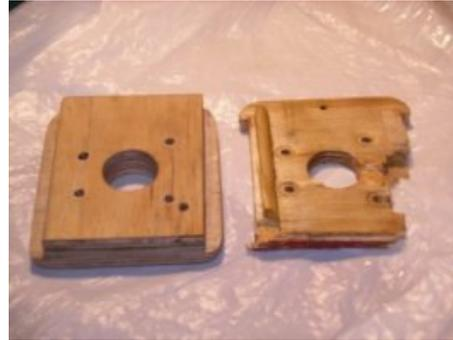
I positioned the fuselage front end on the 7 ply and traced the inside shape and, roughly, the outside shape. Then, for speed, I set up my router to cut to half the depth of the 7 ply and used it to cut out the marked channel. Then a hacksaw quickly freed the embryonic firewall from the rest of the ply offcut. Using the Permagrafit, I fettled the inner edges to fit snugly and squarely into the front of the fuselage.
