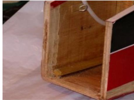
Now is the time to get out the glue! I cleaned up all the surfaces and mixed up the epoxy resin (in my case, you may prefer other glues). I spread the resin generously to the firewall and fitted the reinforcing pieces before checking for squareness and clamping securely in position. When you get to this stage, turn out the lights and walk away!
