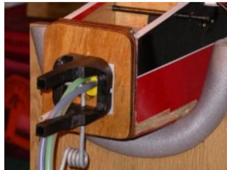
The next photo shows the engine installed with the plumbing completed. The throttle link came from my 'bits' box and was attached (by a ball link) to the carburettor first. The movement of the carburettor control arm was measured and the movement checked against the throttle servo to verify which hole to use for the clevis. I then used my transmitter to set up the throttle as best I could
