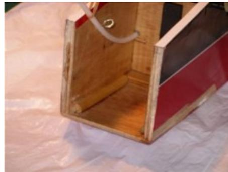
Measuring from the first fuselage former, I estimated that I could achieve a length of 10.5cm (4\14") in front of the former. Measuring along each edge of the fuselage sides from the former enabled a line to be marked on the outside of the body ready for surgery!
