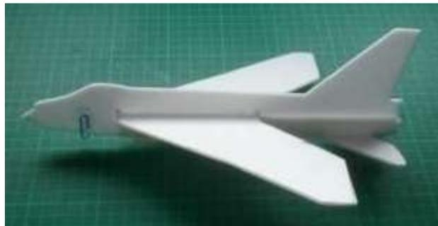
As the CG position is not obvious, I've done some calculations and also made a simple profile 'chuck' glider as a check.
