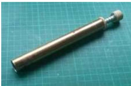
To make all those holes I made a sharpened tube with spring-loaded plunger to quickly get the cut-outs out!
