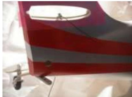
Photo 4 gives a clearer idea of the positioning of the blind nut before dropping. When the blind nut is dropped in, it will slide down the wire when its central pillar will locate in the hole. If it doesn't, shake the wire gently and encourage it into place.
