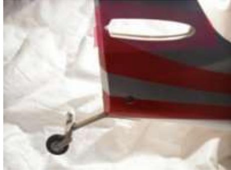
Photo 2. Now rotate the tail wheel bracket away from the centre line and drill out the pilot hole to clear the central pillar of the blind nut. Now the tricky bit; how to get the blind nut into place? My solution was a piece of thin wire pushed up from the bottom and bent out from the tailplane hole.
