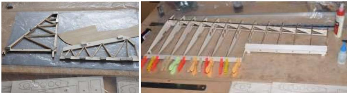
Other than that it went together in a reasonably straight-forward way. The cowl included was of very flimsy plastic, so I made a fibreglass replacement, of which quite a bit had to be cut away to clear the Irvine53. Covering was in red Profilm, and decorations in Solartrim cut to shape on my CraftRobo vinyl cutter.
