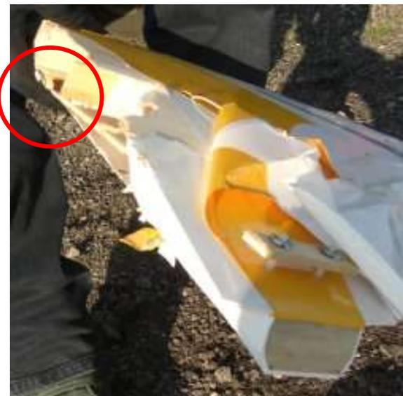
Recently an ARTF model came apart in the air when in level flight with no significant aerobatic loads. An inspection showed that not only was the wing brace little wider than the fuselage, but there was hardly any glue on it.
