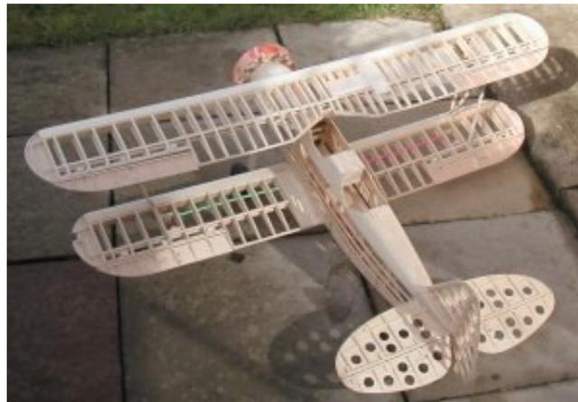
The rigging is elastic cord and is only for scale effect as the wings are very strong, although it does hold the inter-plane struts in place; holes in the ends of the struts engage in wire hooks in the wings and the elastic holds the struts against the hooks.
